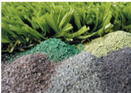
Application of rubber granulate in synthetic turf fields. (Source: Granuband)
