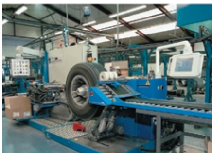
Cold cure retreading: Bandag method. (Source: KARGRO)
